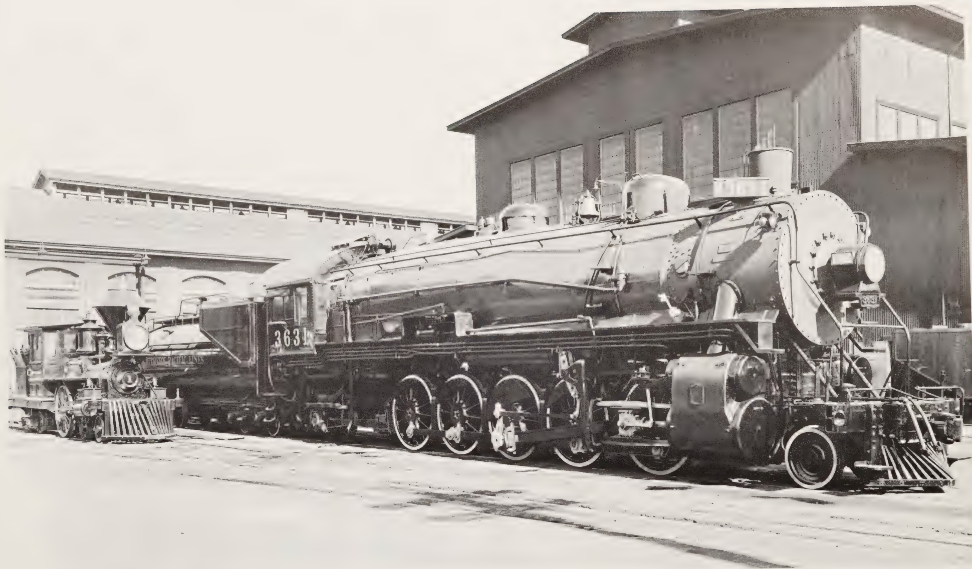
The tiny "C. P. Huntington" Alongside One of the "Prosperity Special" Locomotives. This Veteran Could Almost Fit into the Firebox of the Large Giant Without Choking the Draft.
